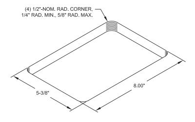
Figure 2- Chassis mounting
